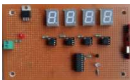
Fig:13. Monitoring circuit board
